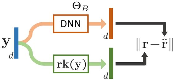
Figure 2: **Training a differentiable sorter.** Given a score vector  $\mathbf{y}$  we learn the parameters  $\Theta_B$  of a DNN such that its output  $\hat{\mathbf{r}}$  approximates the true rank vector  $\mathbf{rk}(\mathbf{y})$ . The model is trained using gradient descent and an  $L_1$  loss. Once trained,  $f_{\Theta_B}$  can be used as a differentiable surrogate of the ranking function.
