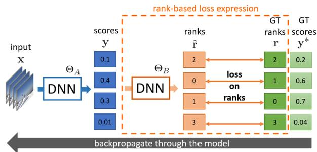
Figure 1: **Overview of SoDeep, the proposed end-to-end trainable deep architecture to approximate non-differentiable ranking metrics.** A pre-trained differentiable sorter (deep neural net [DNN]  $\Theta_B$ ) is used to convert into ranks the raw scores given by the model (DNN  $\Theta_A$ ) being trained to a collection of inputs. A loss is then applied to the predicted rank and the error can be back-propagated through the differentiable sorter and used to update the weights  $\Theta_A$ .
